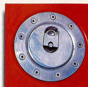
▲ Flush aircraft style fuel cap sits on SFC-style tank. The Palmelli's bespoke parts won't fit a standard Laverda SFC
